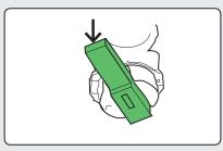
Pull green lever under right side of boiler. Release when indicator on pressure gauge reaches green.
