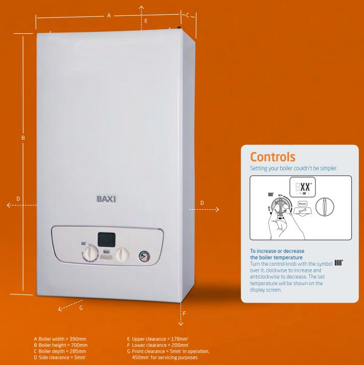
\*These are the minimum recommended clearance dimensions Greater clearance will aid installation and maintenance.
